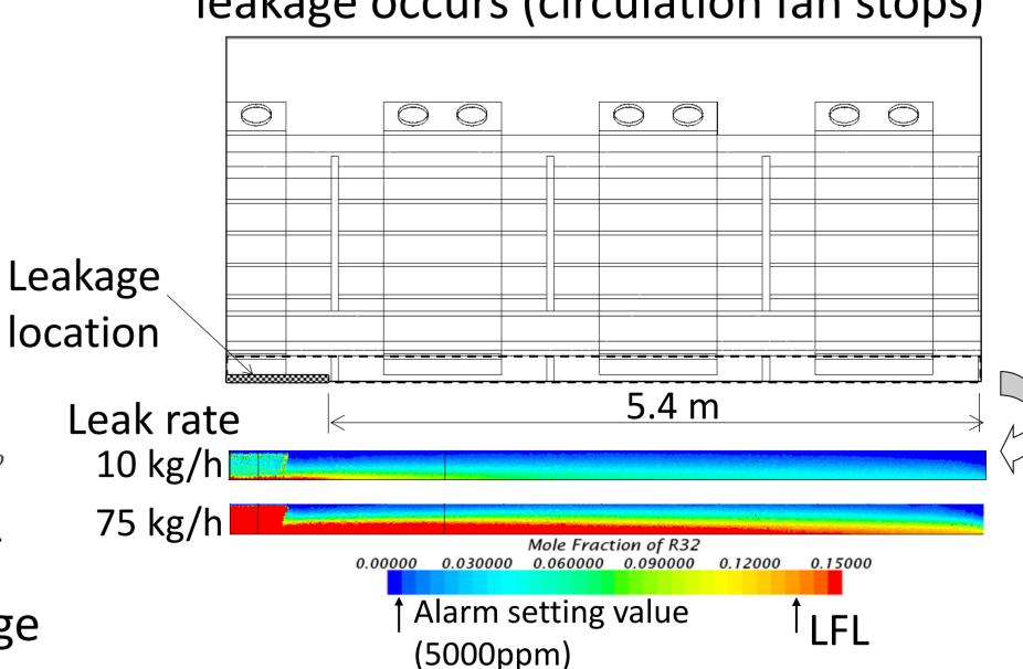
⇒If a detector is within 5 m from the leakage point, it is possible to detect.
