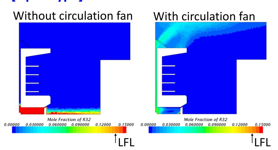
⇒Circulating the refrigerant with a circulation fan, then ensuring safety
