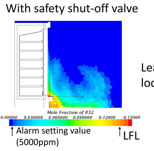
⇒Shutting off the leakage by the shut-off valve, then ensuring safety Concentration distribution when leakage occurs (circulation fan stops)
